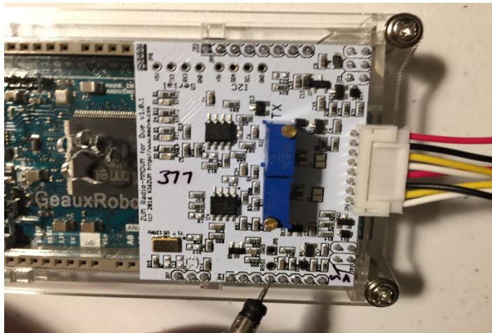
Pin A11 where the probe is touching
